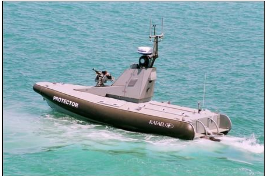
Figure 4: The Protector 9 m unmanned surface vehicle is the only operational combat USV that exists today. The Protector performs surveillance and reconnaissance, as well as force protection duties.
